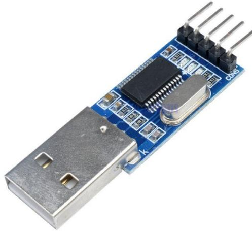
**Figura 4.23:** Conversor TTL a USB
