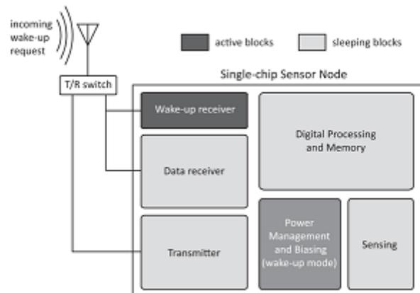
Figure 1. Block diagram of sensor node.
