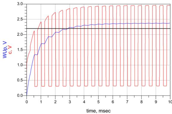
Figure 5. Preamble detector's input (signal 'c') and output (signal 'WUp').
