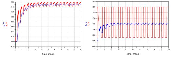
Figure 4. (a) Output from the envelope detector. (b) Adaptive threshold. (c) Output from the comparator, PWM signal.
