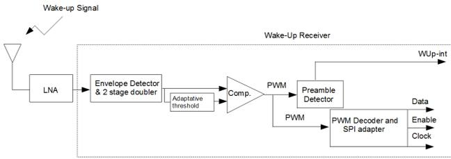
Figure 2. Low Noise Amplifier and Wake-up Receiver Overview.
