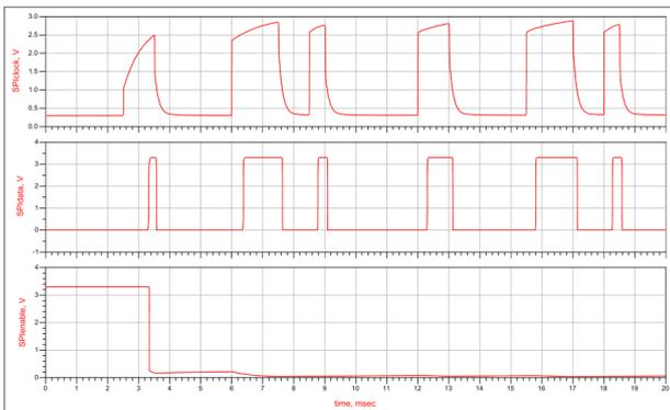
Figure 6. SPI clock, SPI data and SPI enable.
