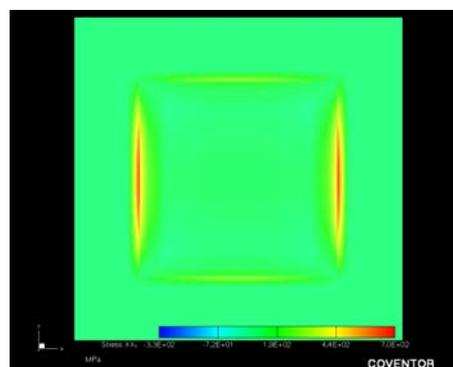
Figure 1: Longitudinal stress profile along X-X'
