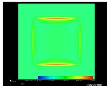
Figure 2: Longitudinal stress profile along Y-Y'
