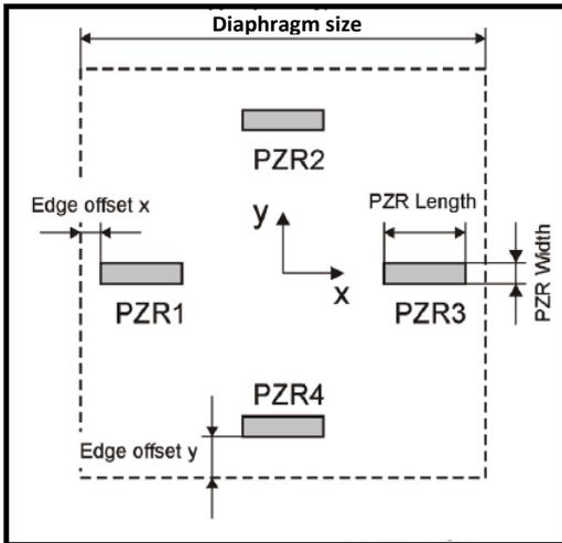
**Figure 3: Piezoresistors in Wheatstone bridge configuration.**
