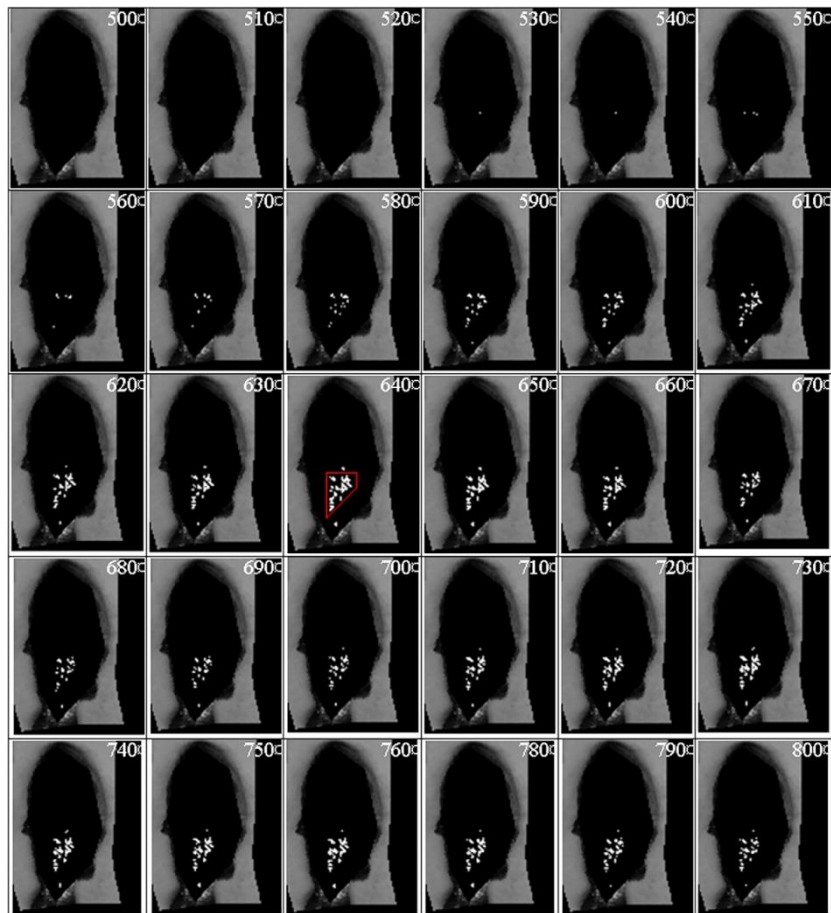
Figure 19. Fish defect detection in VNIR range for each wavelength layer (500 to 800 nm) [33].
